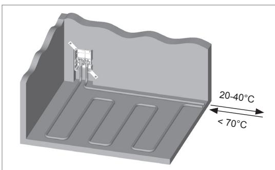
Before starting the plaster work, the RTL head should not be fixed. The protection cover has to be placed on the RTL box. After finishing the wall plastering, remove the protection cover, connect the RTL head, fix the box cover and finally the plastic ring.
