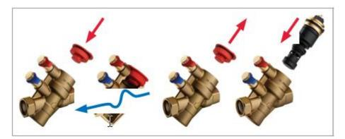
When the system flushing is completed, all filters and strainers have to be cleaned, the pre-setting cap is removed and the cartridge is inserted into the valve housing again and tightened carefully.
